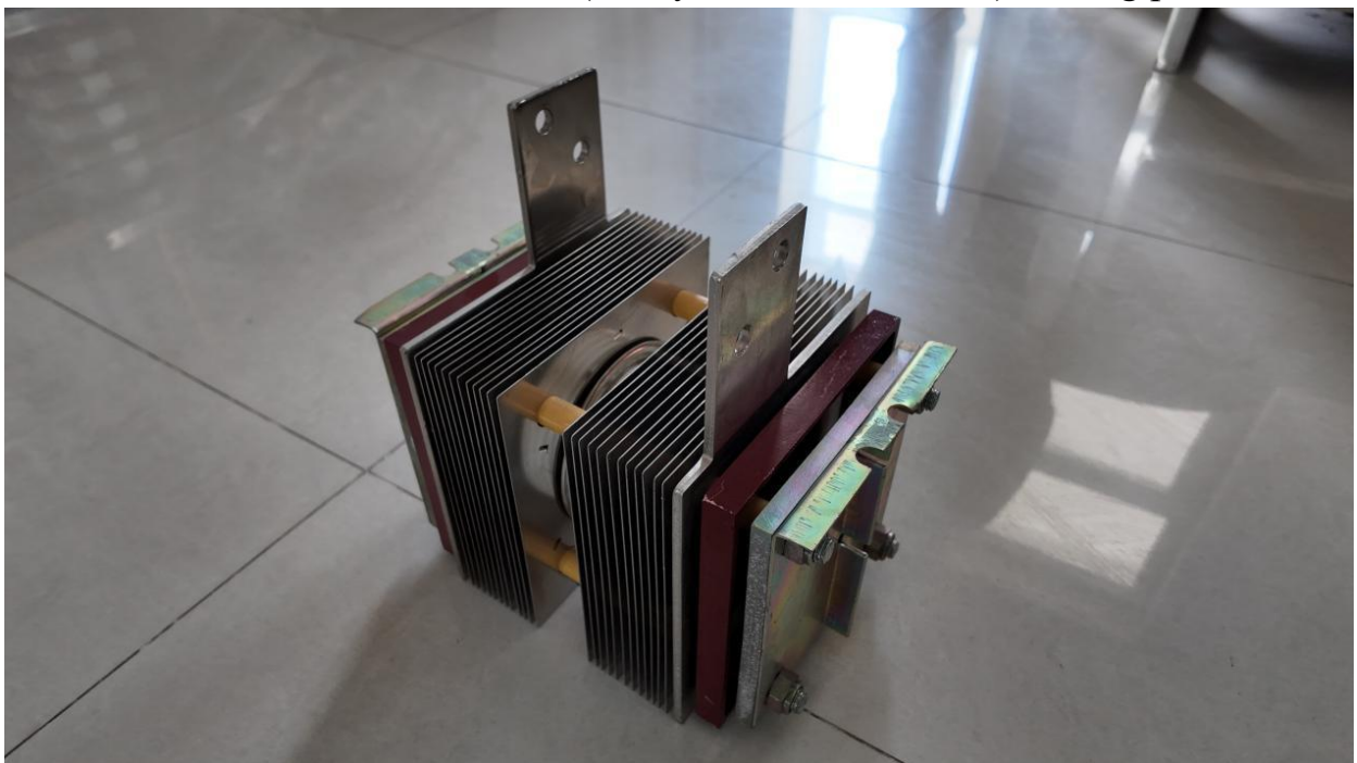
Figure 7 Retrofitted thyristors and diodes with heat sinks
